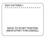
Use the joystick or arrow keys to move the camera view to the appropriate starting position for the pattern, and set the desired zoom.
